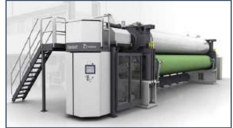
Metso's papermaking equipment. The machine's calender is controlled by a digital hydraulic system.
