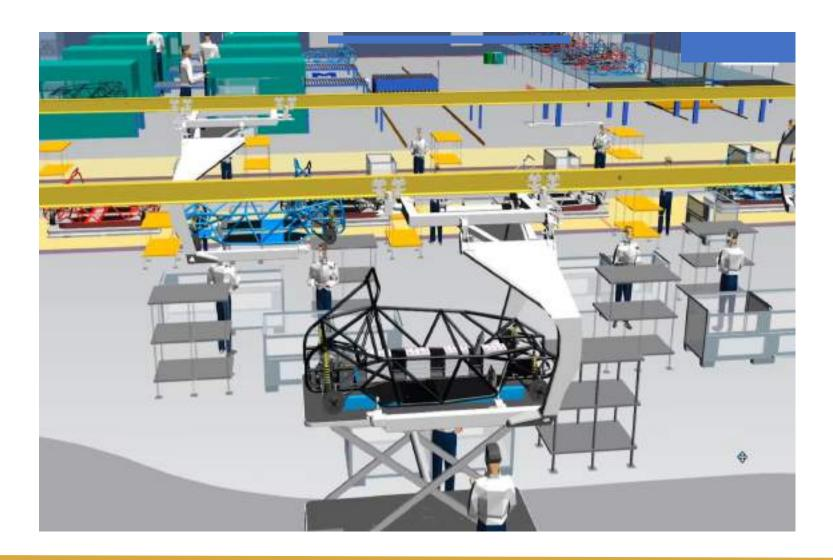
Plan, simulate, predict and optimize production digitally with PLC code generation and virtual commissioning
